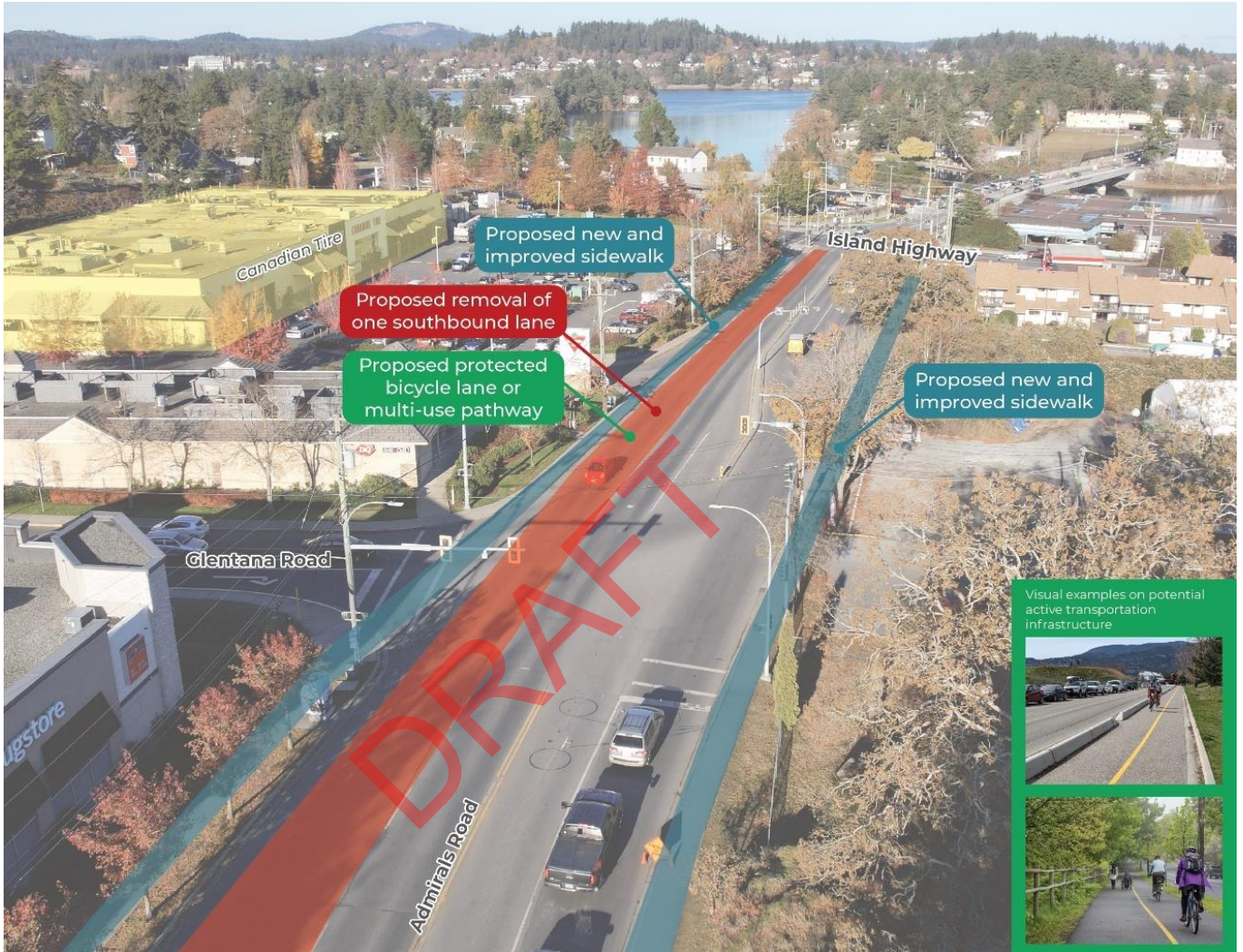
Figure 7. Proposed Improvements on Admirals Road Corridor
